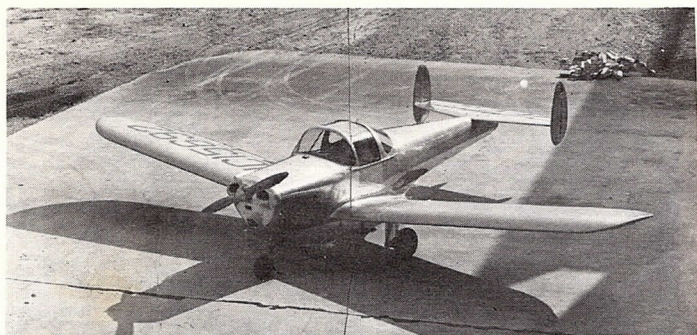
NC15692 in its final form. A wind generator and trailing antenna under the center section. Antenna top rear cockpit to the tops of the tails. No oil cooler. The prop has a flaired hub with an aluminum ring flaring into the nose bowl. The nose bowl has checks at the cylinder air opening.
