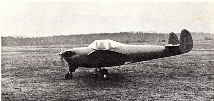
The first of the double tails. Notice the nose gear fairing and side windows. There is a lump in the center leading edge of the horizontal tail. I haven't been able to find out what it is and they went back to the short wing fairing.
