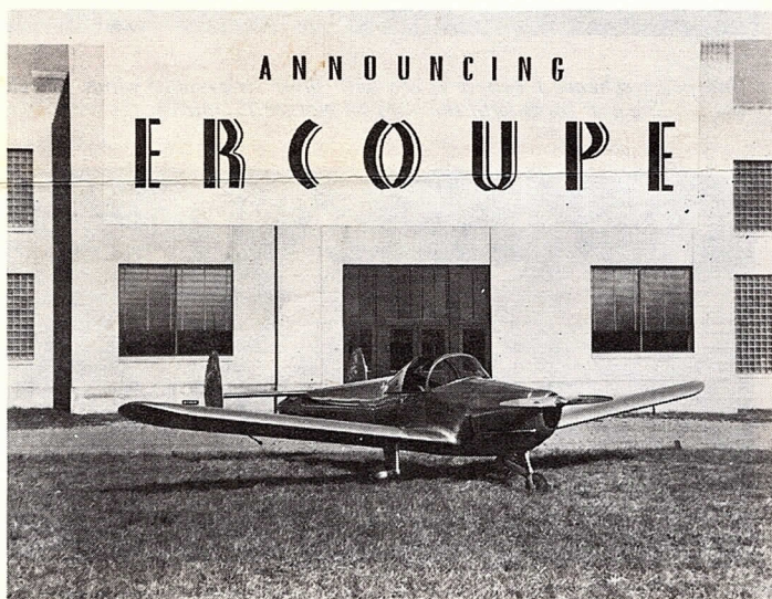
The first production NC15692. The gear legs are different from the prototype photo No. 7. External aileron counter weights, polished aluminum finish fuselage, red numbers, silver wing. This picture is a promotion ad.
